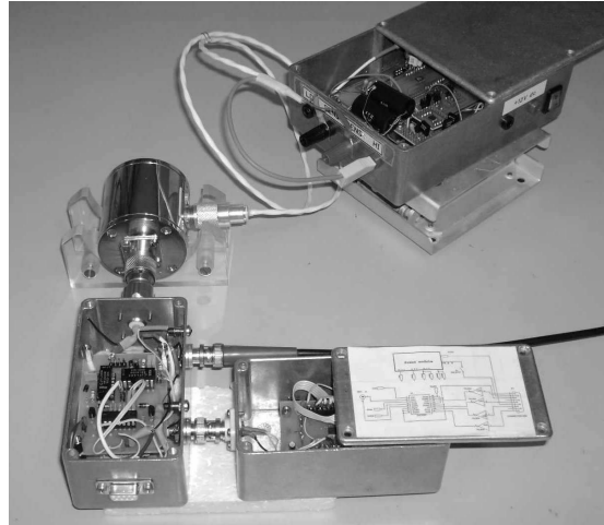
Fig. 2. First implementation of the system for precise measurements of RMS voltages suitable for preliminary tests.
